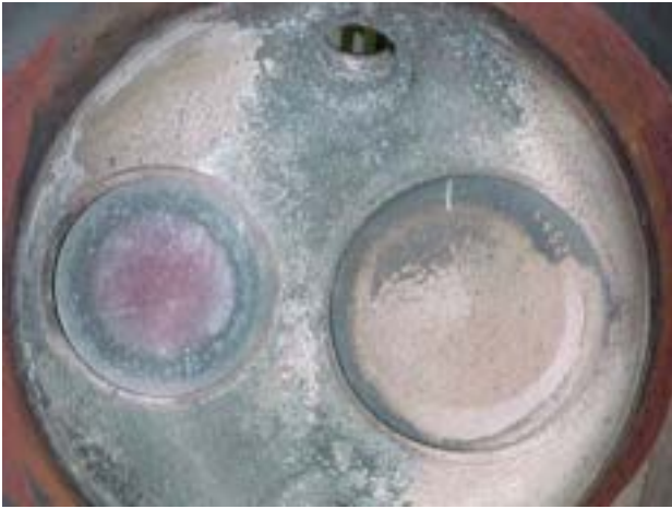
Normal Combustion Chamber. Exhaust valve has reddish combustion deposit in center with dark outer edge. Intake valve has light brown combustion deposits. Combustion chamber has light brown deposits.
